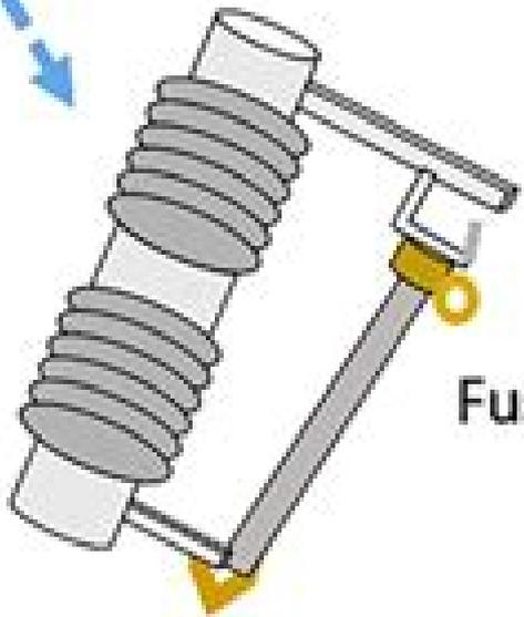
Fuse\* Note: Fuse is tripped and closed without relay, which is widely used for lateral branch protections.
